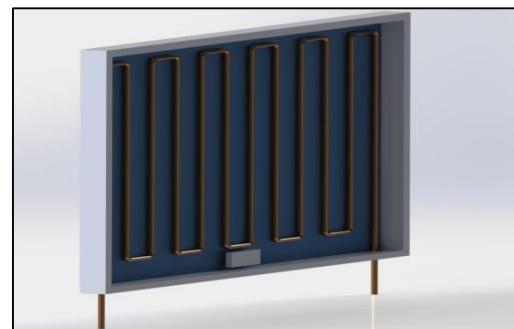
Gambar 2. Hybrid photovoltaic thermal (PV/T)
