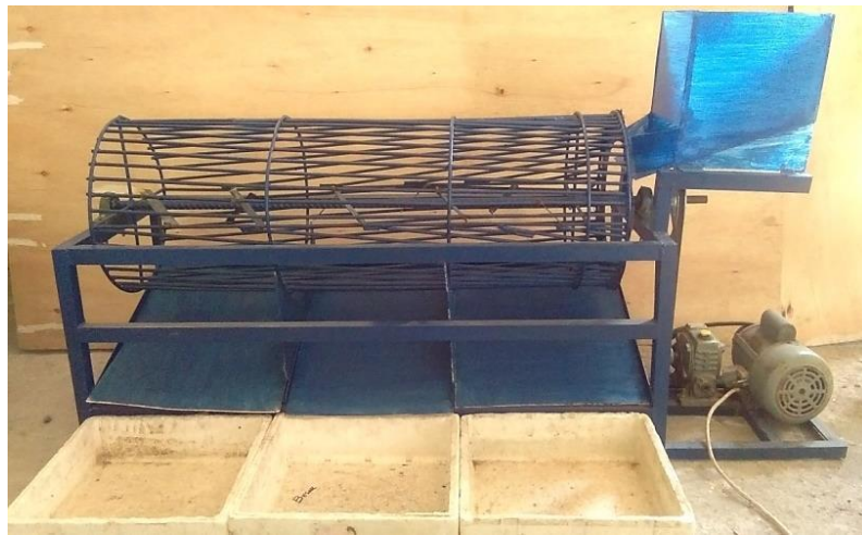
Figure 4. Prototype of the palm seed sorting machine.
