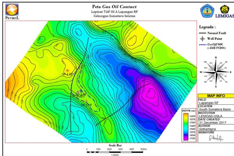
Gambar 9. Pemodelan Peta GOC lapisan TAF-SS-A (-1328m TVDSS)
