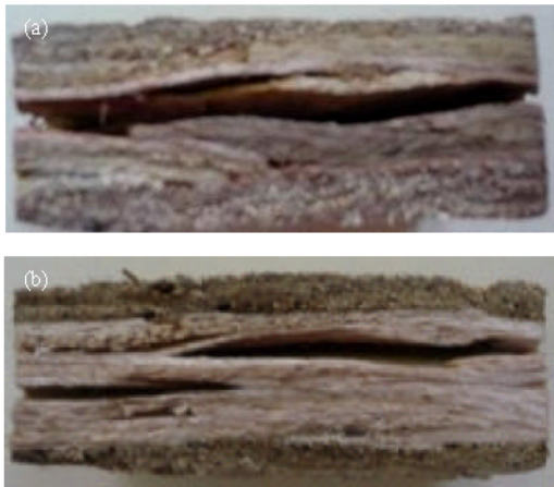
Fig. 7: Internal bond failures in the boards; (a) Steeper density profile and (b) uniform density profile
