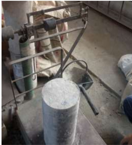
Fig 5. Measuring the specimen weight
