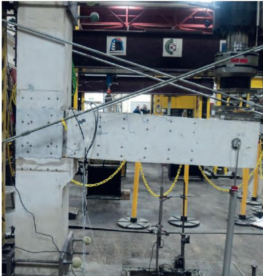
Fig. 6: Crack pattern of beam-column specimen subjected to static-monotonic loading (Specimen P1)
