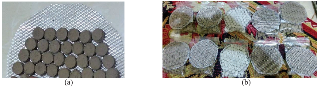
FIGURE 1. (a) Zeolite/coal-fly ash pellets and (b) the pellet filters.
