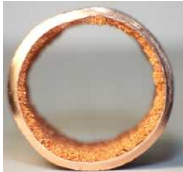
Gambar 7. Sintered powder wick tembaga [19]
