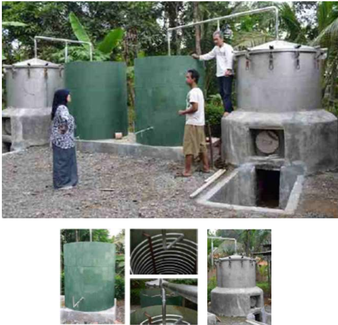
Fig. 2. Liquid smoke of coconut shell production apparatus (Margiwiyatno et al. , 2013).
