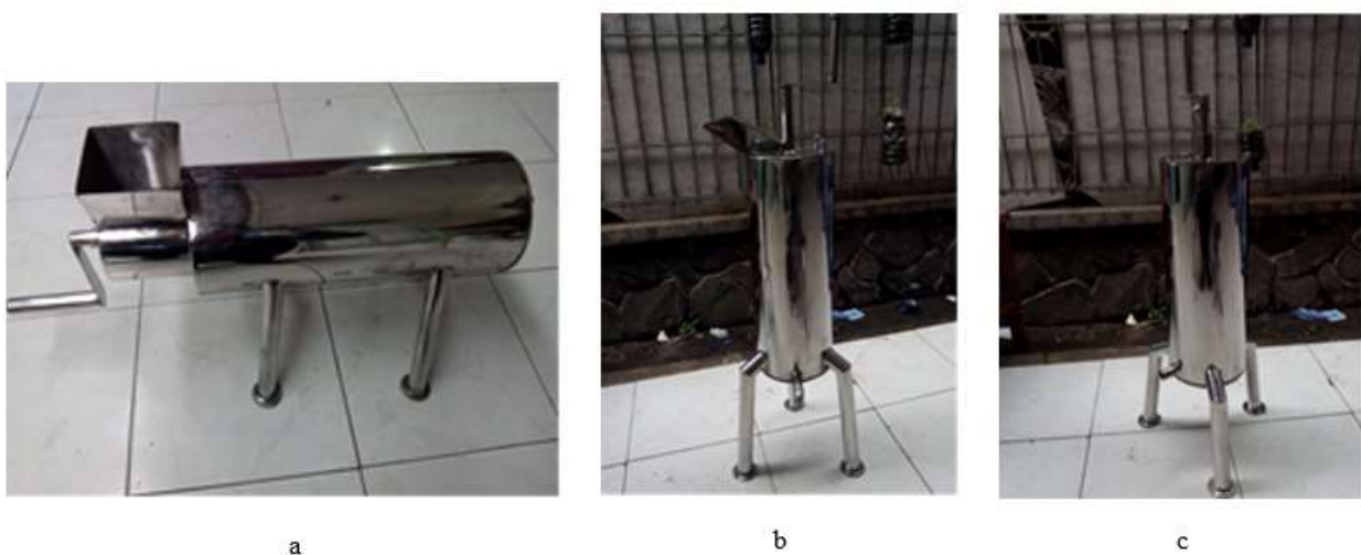
Fig. 1. Mechanism of separation a) horizontal brush rotating mechanism, b) vertical mechanism with rotary brush, and c) vertical mechanism with static brush
