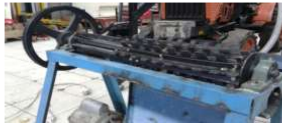
Fig. 2 .The Cylinder of Corn Sheller
