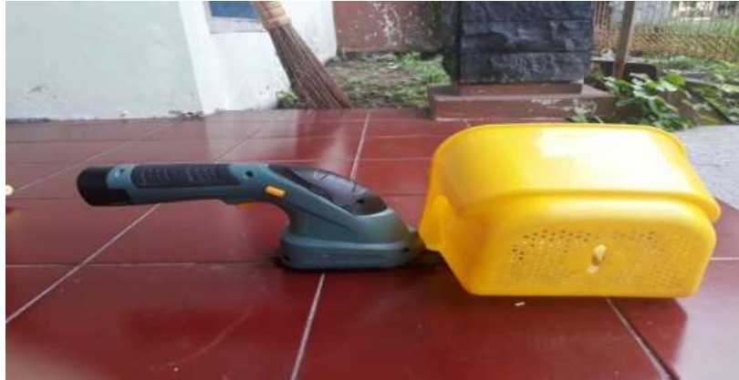
Fig. 2. Tea Picking Machine Reciprocating Types With A Battery Power Source E-Tem M01 7,2 Volt 3000 mAh Collection Box
