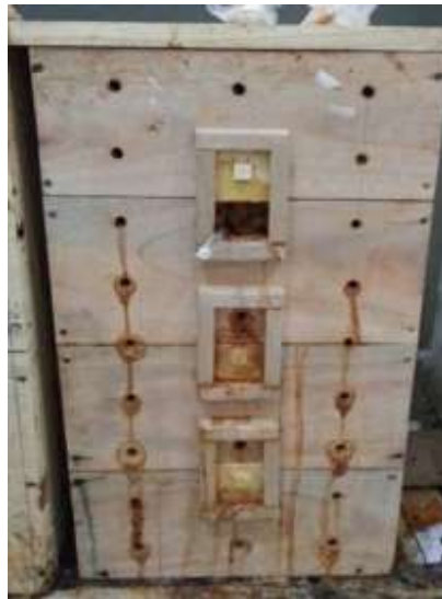
Fig. 1. A small fermentation box (26 x 20 x 45 cm)
