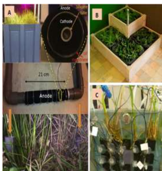
Fig 4. Three types of P-MFC models; A. Tubular, B. Modular, and C. Flat plat (source: Wetser (2016) and plant-e.com)
