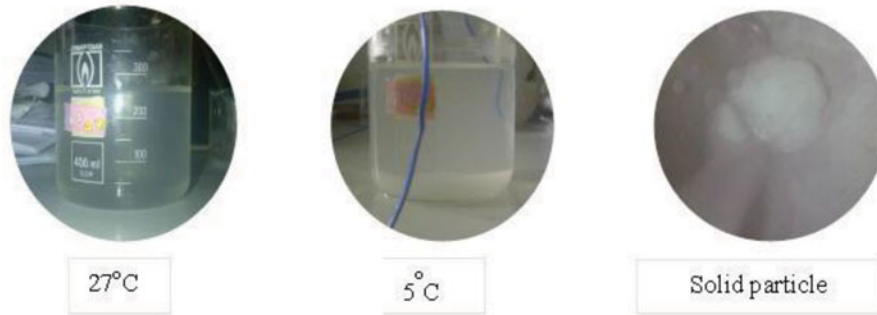
Fig. 4. Visualization of salt hydrate from Na 2 HPO 4 3.6% mass fraction.
