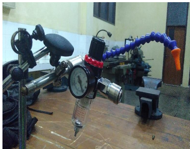
Figure 2. Vortex tube used to produce air cooling.
