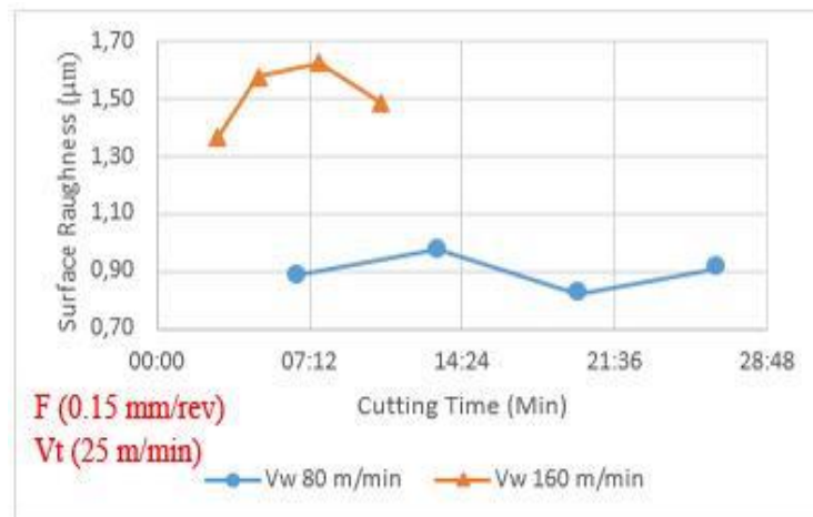
Figure 7. Graph speed the workpiece ( V_w ) of the surface roughness values.
