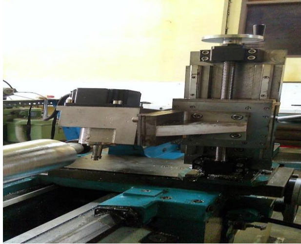
Figure 1. Rotary cutting tool system
