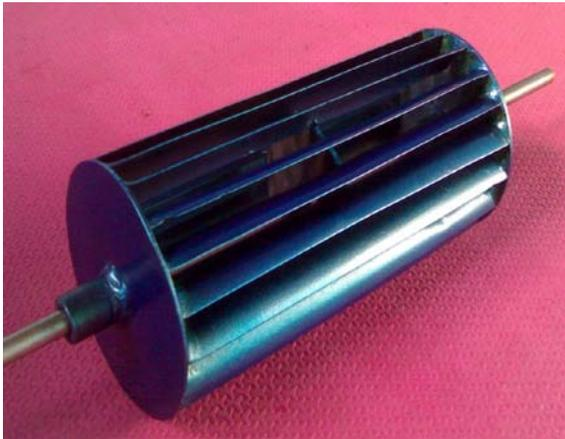
Gambar 10. Model turbin aliran silang (*cross flow*)
