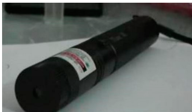
Figure 2. Photograph of a green laser pointer charge 303 with the following specifications: surface treatment, black anodized; battery, lithium 18650; max output, <3 W; working voltage, dc 3.7 V.
