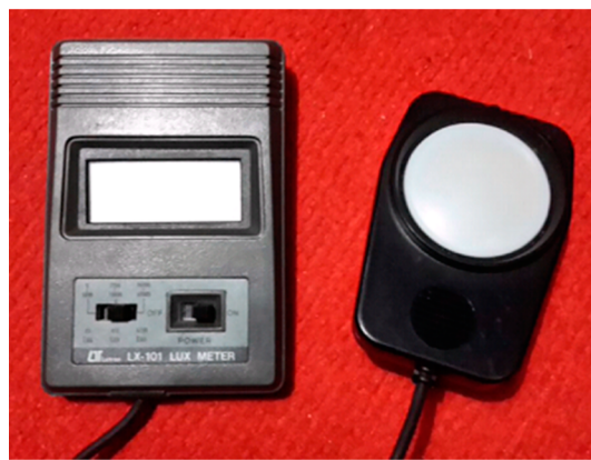
Figure 3. Photograph of a lux meter lutron LX-101. Specifications follow: ranges, 0–50,000 lux, three ranges; zero adjustment, internal adjustment; sampling time, 0.4 s; sensor structure, the exclusive photodiode and color correction filter; operating temperature, 0–50 °C; power supply, dc 9 V battery, 006P, MN1604 (PP3), or equivalent; power consumption, approximately dc 2 mA.
