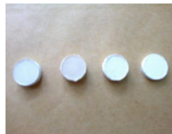
Figure 2. Typical Examples of Sodium Carbonate Pellets after Calcined at 110\text{ }^\circ\text{C}
