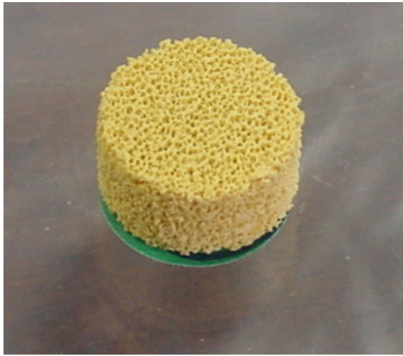
Figure 1. Ceramic foam monolith loaded with a catalyst.
