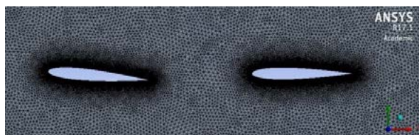
Fig 4. Example of numerical model for stagger 2-c
