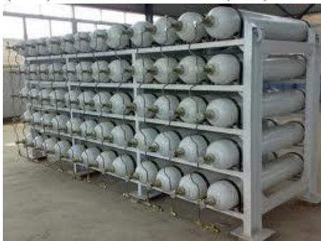
Figure 4. pressure of 200 bar CNG Tubes
