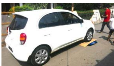
Figure 10 Weighing the car in a flat position
