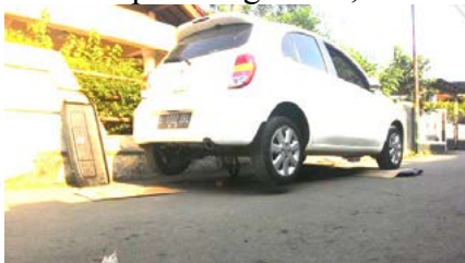
Figure 11 Weighing the car in a sloping position
