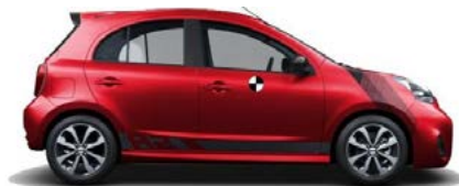
Figure 12 Approximate position of CG on car
