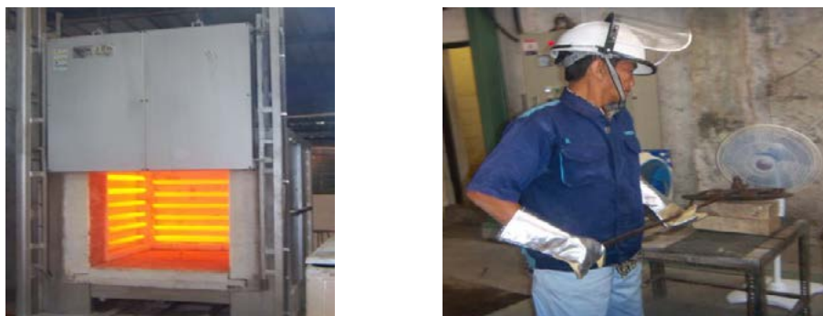
Figure 2. The heat treatment process of manufacturing track link tank
