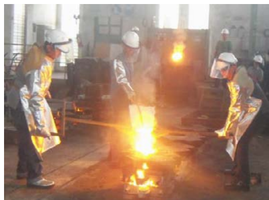
Figure 1. The casting process of manufacturing track link tank
