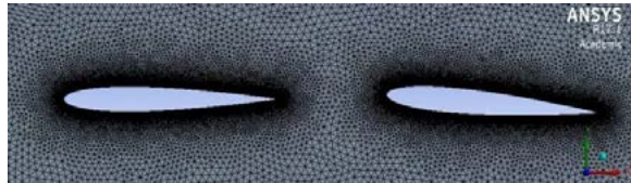
Fig 3. Example of numerical model for stagger 1.5-c
