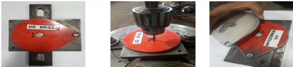
Figure 10. Drilling process using jig (after improvement)
