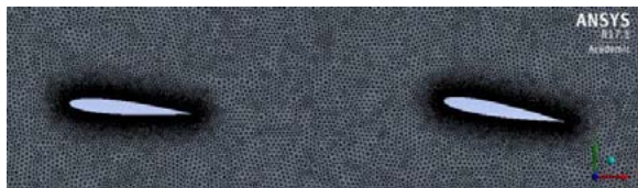
Fig 5. Example of numerical model for stagger 3-c
