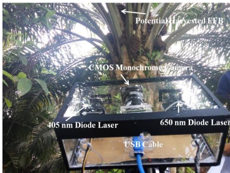
Figure 2. LIFI System on tripod 2 m from a 3 m oil palm tree.
