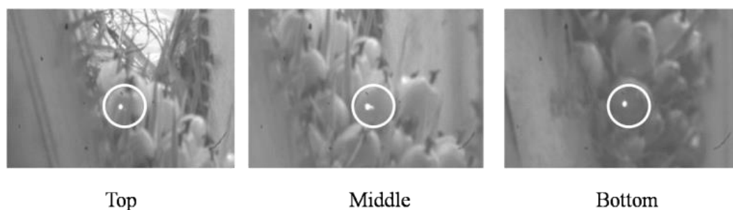
Figure 3. Images of fruit illuminated by 650 nm laser spot for three parts of an on-tree oil palm FFB
