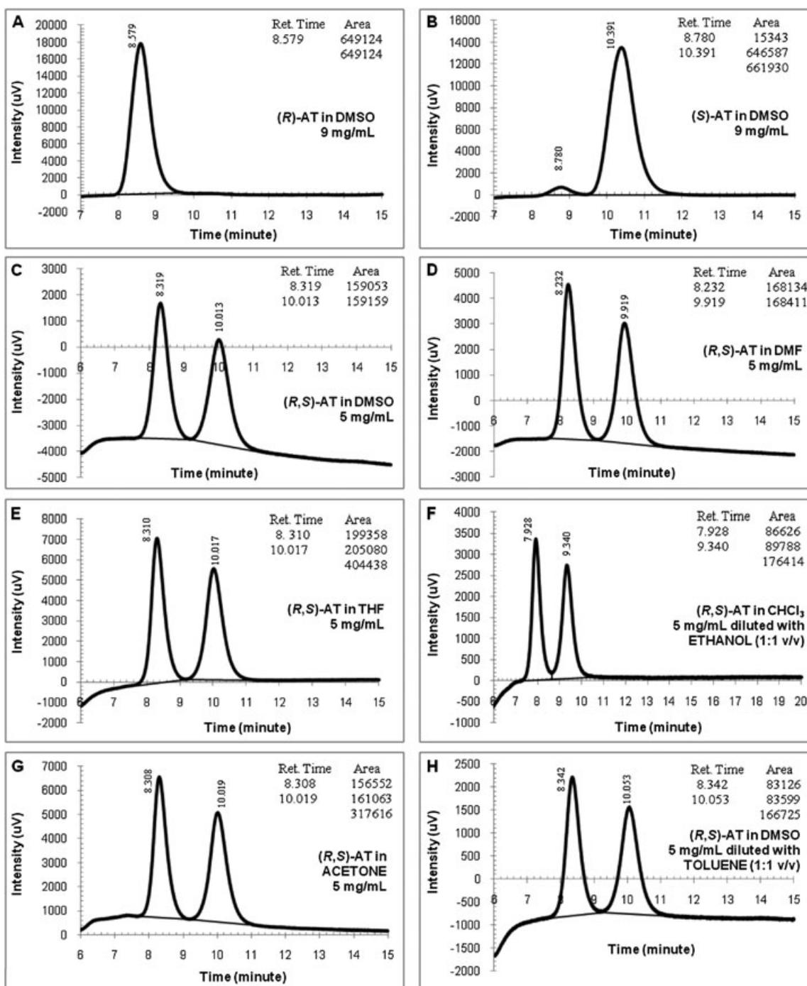
**Fig. 3.** Chromatograms of the atenolol (AT) in organic media (conditions: 254 nm, 35 °C, 1 ml/min; injection volume: 2 µl; centrifuged samples). (A) (R)-AT in dimethyl sulfoxide (DMSO), (B) (S)-AT in DMSO, (C) (R, S)-AT 5 mg/ml, (D) (R,S)-AT in dimethylformamide (DMF), (E) (R,S)-AT in tetrahydrofuran (THF), (F) (R,S)-AT in CHCl<sub>3</sub> 5 mg/ml diluted with ethanol (1:1 v/v), (G) (R,S)-AT in acetone 5 mg/ml, and (H) (R,S)-AT in DMSO 5 mg/ml diluted with Toluene (1:1 v/v).
