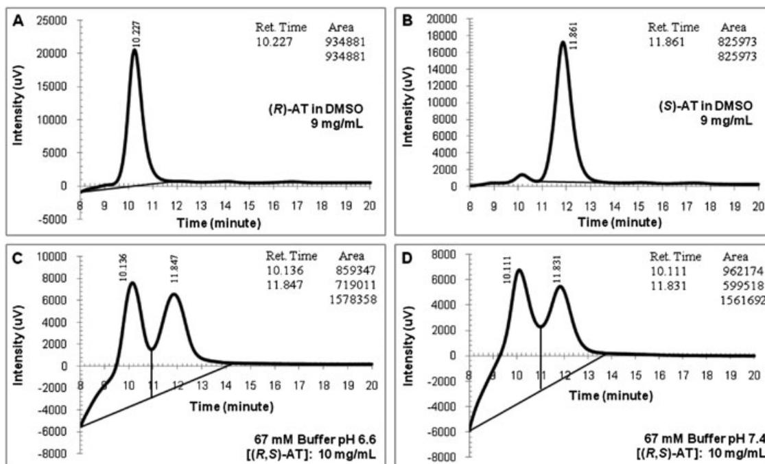
**Fig. 5.** Representative peaks of atenolol (AT) dissolved in dimethyl sulfoxide (DMSO) and Sorensen buffers (conditions: 254 nm, 35 °C, 0.75 ml/min; injection volume: 2  $\mu$ l; centrifuged samples). (A) (*R*)-AT in DMSO 9 mg/ml, (B) (*S*)-AT in DMSO 9 mg/ml, (C) 67 mM buffer pH 6.6 [(*R,S*)-AT]: 10 mg/ml, and (D) 67 mM buffer pH 7.4 [(*R,S*)-AT]: 10 mg/ml.
