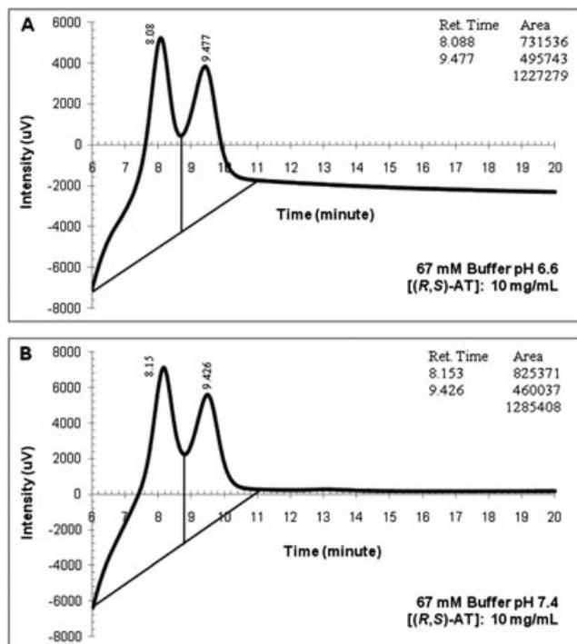
**Fig. 4.** Chromatographic diagrams of atenolol (AT) dissolved in Sorensen buffers (conditions: 254 nm, 35 °C, 1 ml/min; injection volume: 2  $\mu$ l; centrifuged samples). (A) 67 mM buffer pH 6.6 [(*R,S*)-AT]: 10 mg/ml and (B) 67 mM buffer pH 7.4 [(*R,S*)-AT]: 10 mg/ml.
