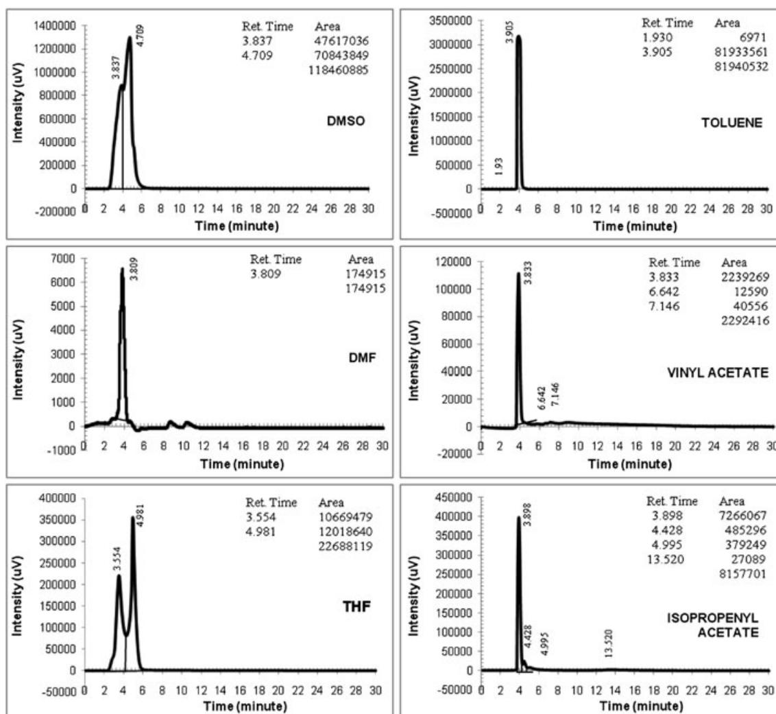
Fig. 2. Representative peaks of the experimental solvents (conditions: Protocol-01, 254 nm, 35 °C, 1 ml/min flow rate; injection volume: 5  $\mu$ l; filtered samples). DMSO, dimethyl sulfoxide; DMF, dimethylformamide; THF, tetrahydrofuran.
