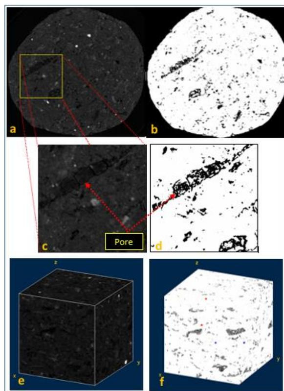
**Figure 3.** Digital rock physics was processed of sandstone. (a) 2D original image (gray scale), (b) image made in thresholding, (c) sub-cube from the original image, (d) threshold image from c, (e) 3D image from c by dimension  $300 \times 300 \times 300$  pixels, and (f) 3D threshold image from e.
