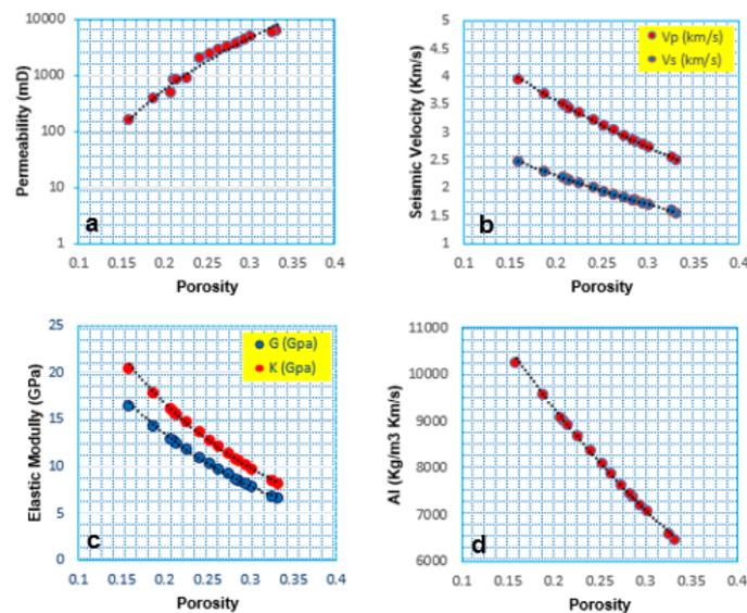
**Figure 4.** The calculation of permeability and elastic properties of sandstone sample. (a) estimation of permeability, (b) estimation of  $V_p$  and  $V_s$ , (c) estimation of Bulk modulus and shear modulus, and (d) estimation of acoustic impedance.
