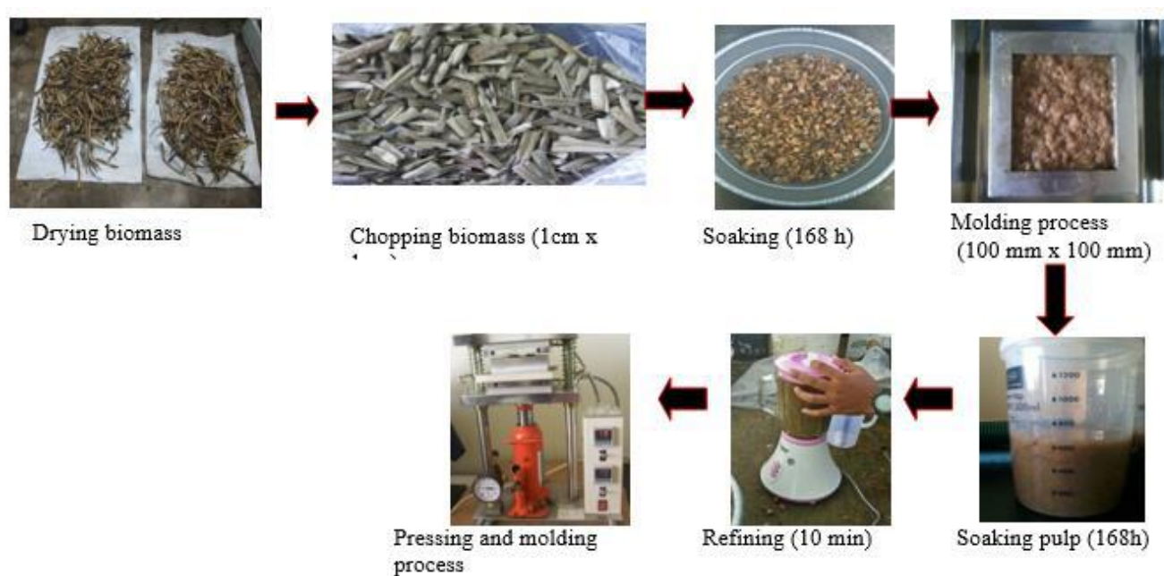
Fig 1: Biodegradabel board producing process
