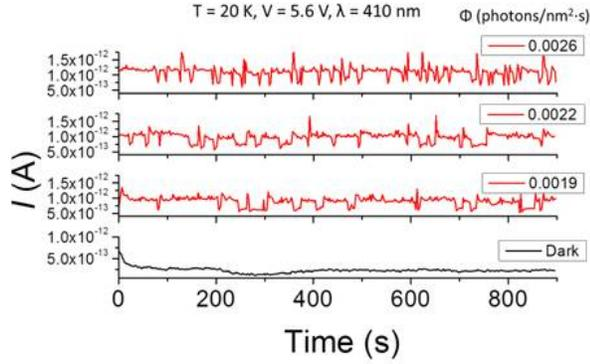
Fig. 3.  $I$ -time characteristics in dark and under light illumination. Under light illumination, current switch between two or more levels. By increasing incident photon flux ( $\Phi$ ), from bottom to up, number of RTS increases, suggesting that current jumps are triggered by photons [16].
