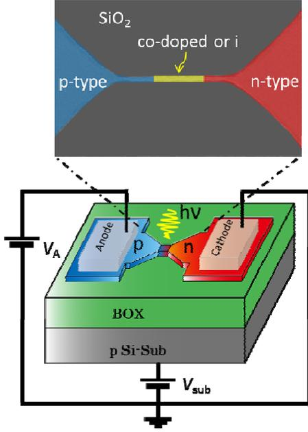
Fig. 1. Schematic device structure, bias configuration and schematic top view of  $p$ - $n$  and  $p$ - $i$ - $n$  junction area.
