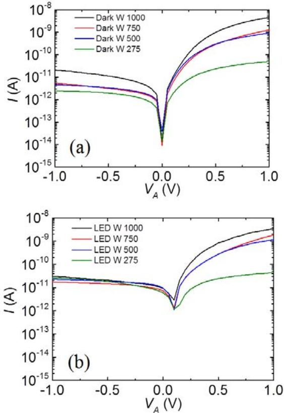
Fig. 5.  $I$ - $V_A$  characteristics of  $p$ - $n$  junction devices in (a) dark and (b) under LED illumination for several devices with different channel width. Under LED illumination, narrow channel-width devices show higher photosensitivity.
