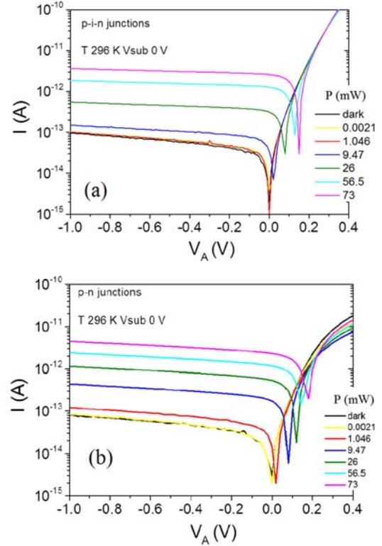
Fig. 4. Typical room temperature  $I$ - $V_A$  characteristics of (a)  $p$ - $i$ - $n$  and (b)  $p$ - $n$  junctions in dark and under light illumination. Both devices show photovoltaic effect under halogen light illumination, i.e., reverse current increases by increasing photon flux.
