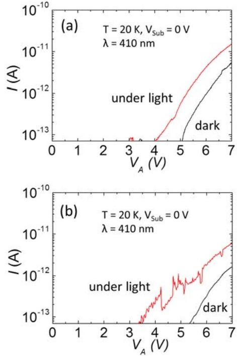
Fig. 2. Low temperature  $I$ - $V_A$  characteristics of (a)  $p$ - $i$ - $n$  devices and (b)  $p$ - $n$  junction devices. Only  $p$ - $n$  junction devices show noise feature under light illumination [16].
