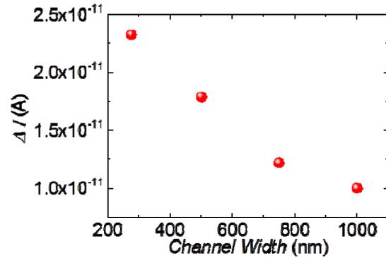
Fig. 6. Current enhancement ( $\Delta I$ ) due to light illumination for several devices with different channel-width. Narrow devices have larger  $\Delta I$  indicating that they are generating current from photons efficiently.
