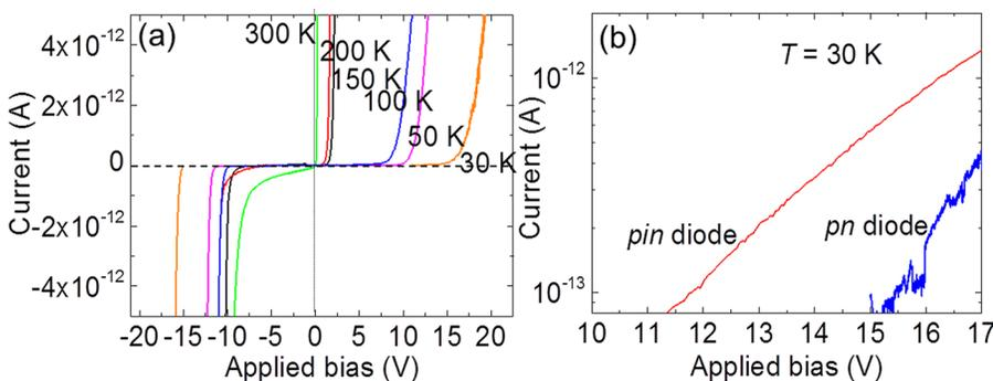
FIG. 2. (a) Temperature dependence of *I-V* characteristics for a *pn* diode under reverse and forward bias. (b) *I-V* characteristics of a *pn* diode and a *pin* diode at low temperature ( $T = 30 \text{ K}$ ) under forward bias.
