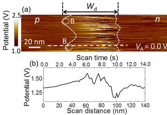
FIG. 5. (a) Electronic potential landscape measured by low-temperature ( $T = 15$  K) KFM across a  $pn$  junction's depletion region. The depletion region is delineated by white dashed boundaries. B dopants are schematically shown at the boundary. (b) Line profile illustrating potential fluctuations as a function of both scan distance and scan time.
