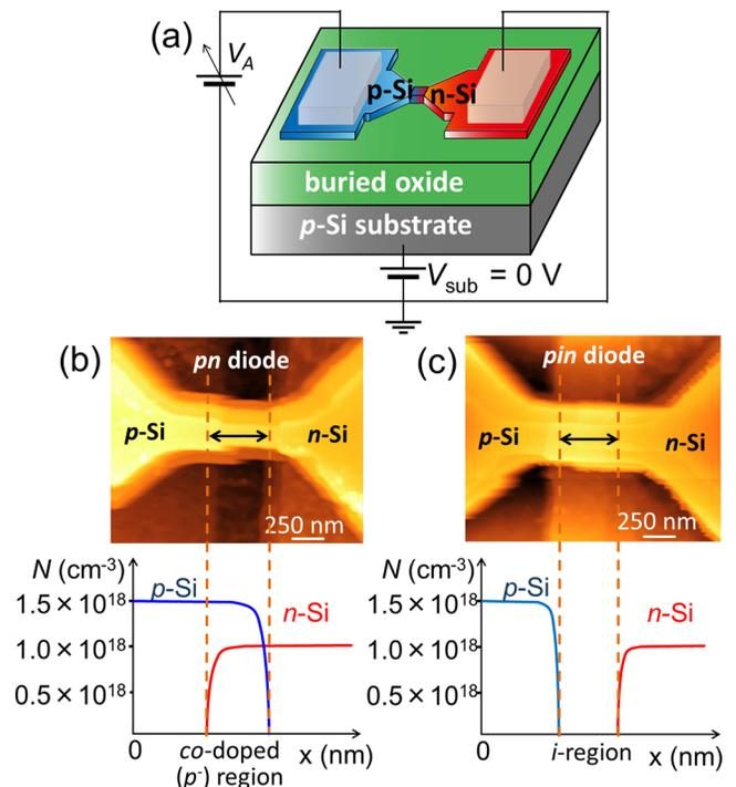
FIG. 1. (a) Device structure of a  $pn$  diode and measurement setup. (b), (c) AFM images and doping concentration profiles for  $pn$  junctions (containing a co-doped region) and  $pin$  junctions (containing an intrinsic region).
