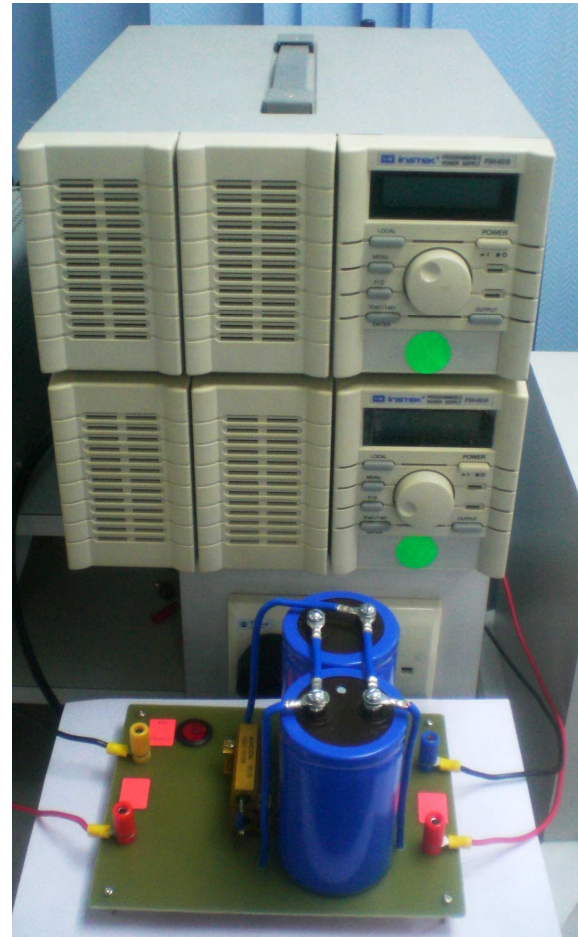
Figure 3. Photograph of PEM fuel cell emulator
