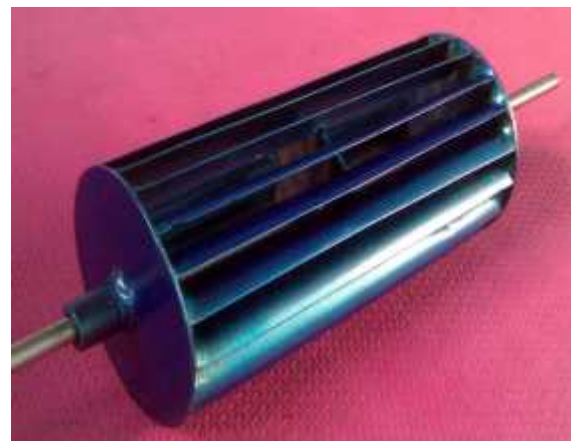
Gambar 10. Model turbin aliran silang ( cross flow )
