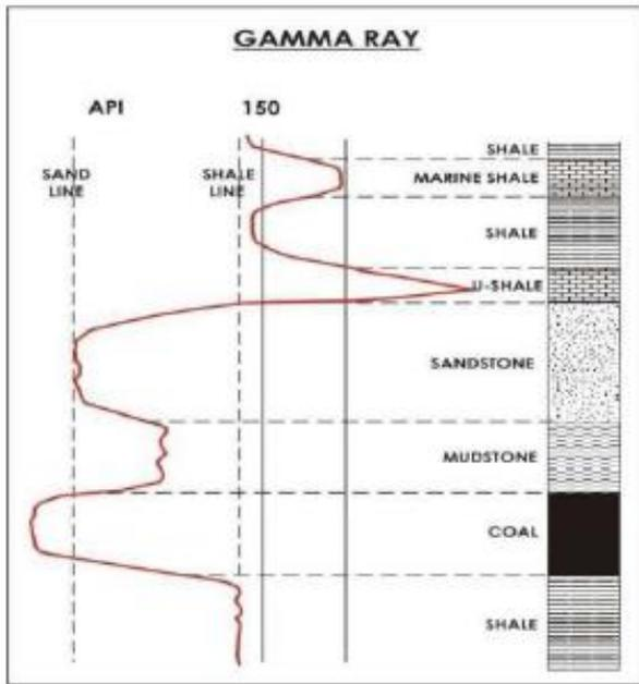
**Gambar 4.** Penentuan Penarikan Sand Base Line dan Shale Base Line (BPB Manual, 1981).
