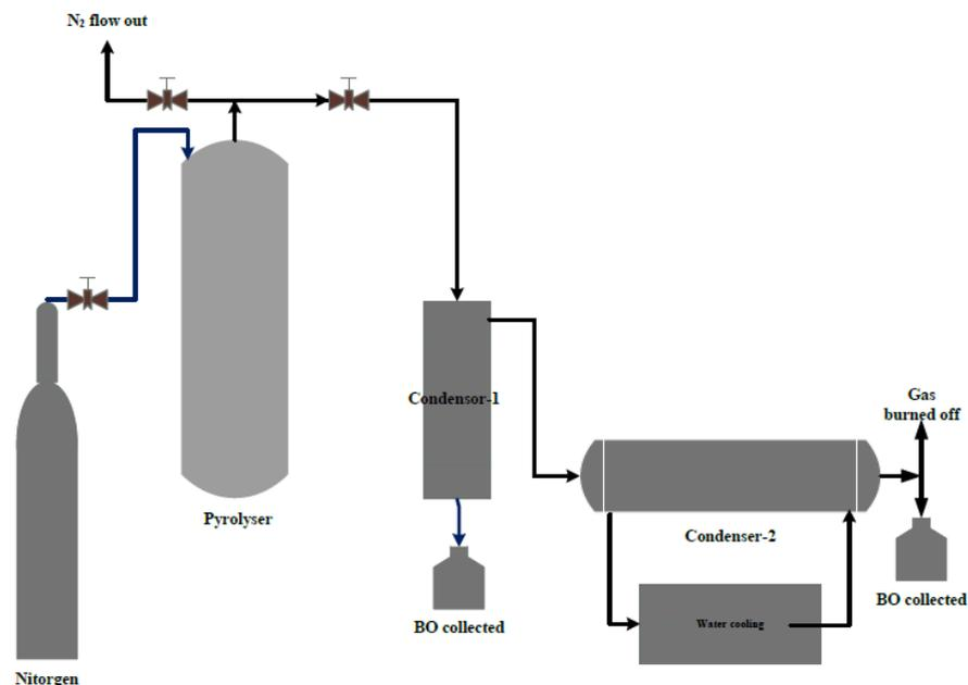
Fig. 3. The installation of experiment apparatus
