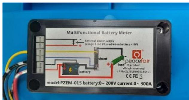
Gambar 4. Multifunctional Battery Meter
