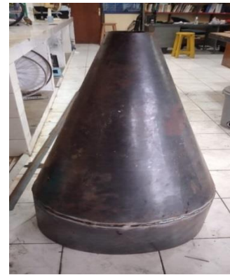
Figure 7. Fabricated Conical Basin.
