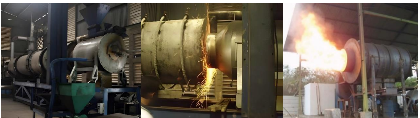
Figure 3. Cyclone burner ( Monika & Suprpto, 2011 )
