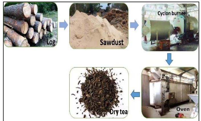
Figure 2. Drying tea leaves using cyclone burner technology fueled by wood sawdust
