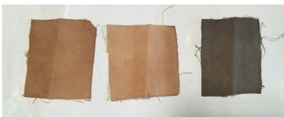
Figure 7. The final fixation color of the dyed cotton cloth (a) lime; (b) alum; (c) ferrous sulfate
