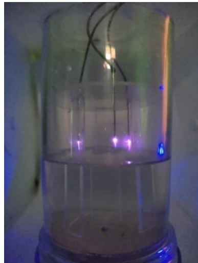
FIGURE 4. Treatment process by applying pulsed field electric above the sample surface.
