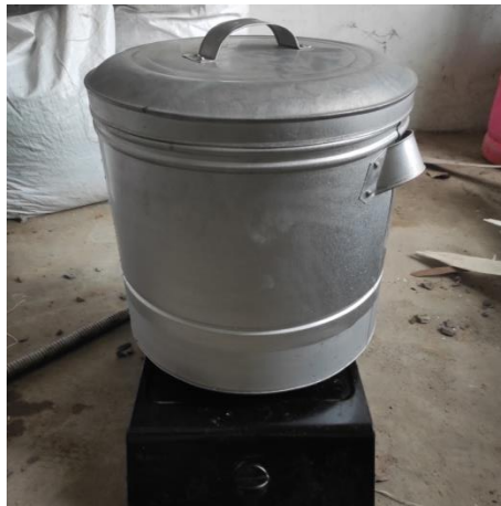
FIGURE 1. Curing treatment by boiled water steam in a tank
