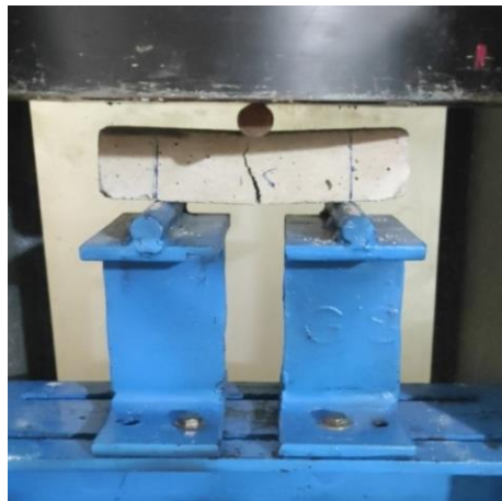
FIGURE 2. Flexural test with three points loading on a prism
