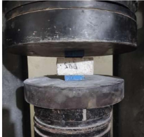
FIGURE 3. Compression test on part of prism
