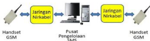
Gambar 1. Mekanisme Store and Forward
