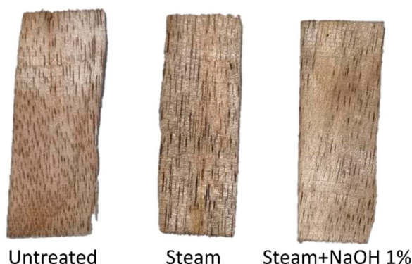
Figure 2. Appearance of sengon strands at various pretreatments.
