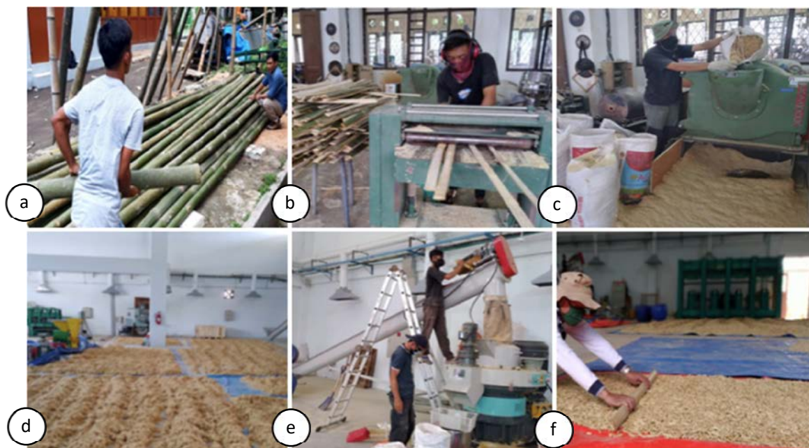
Fig. 1: The process of producing bamboo pellets: (a) Raw materials used; (b) The process of removing the outer and inner skin layers of the bamboo; (c) The production process of transforming the bamboo into its powdered form; (d) Drying the bamboo powder; (e) Producing pellets using the pellet mill; (f) Cooling and conditioning process after pelletization.
