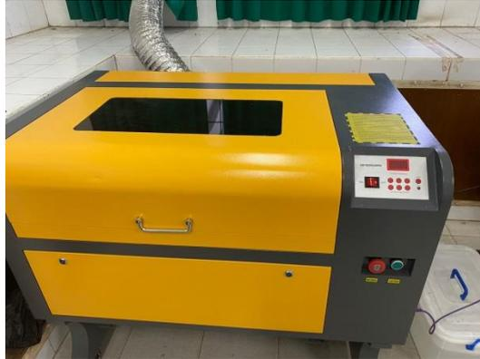
Gambar 2. Mesin laser CO<sub>2</sub>CNC LS-6040 50 Watt.
