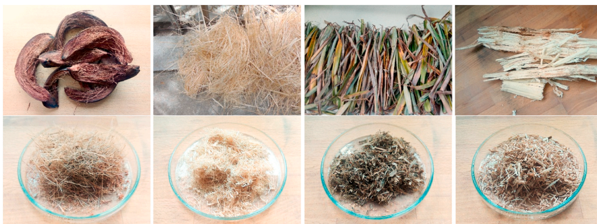
Fig. 2. Investigated material samples before and after processing: a) coconut mesocarp fibre (CF), b) bamboo skin (BS), c) pineapple leaves (PL), d) sugarcane bagasse (SB).
