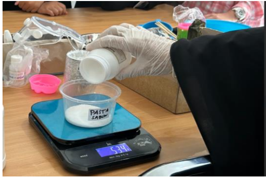
Gambar 2 Proses Penimbangan NaOH dan aquadest
