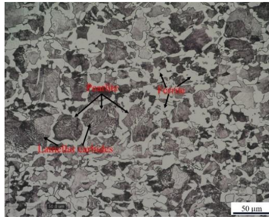
FIGURE 4. Optical microstructure of AISI 4140 steel in annealing condition
