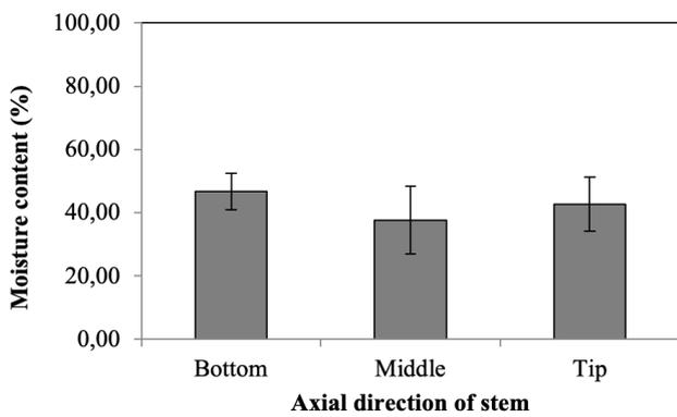
Figure 5. The moisture content of Simalambuo wood
