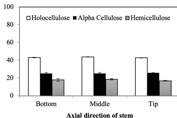
**Figure 10.** Holocellulose, α-cellulose, and hemicellulose of Simalambuo wood
