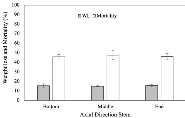
Figure 12. Weight loss and mortality of Simalambuo wood
