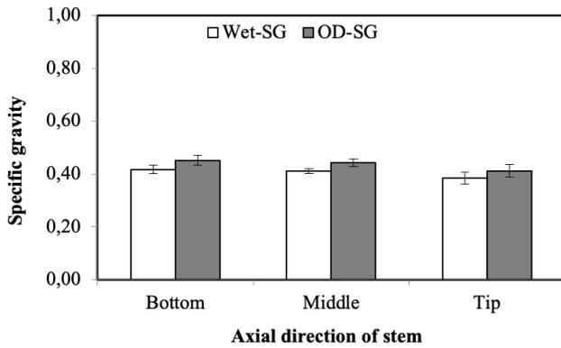
Figure 4. The specific gravity of Simalambuo wood
