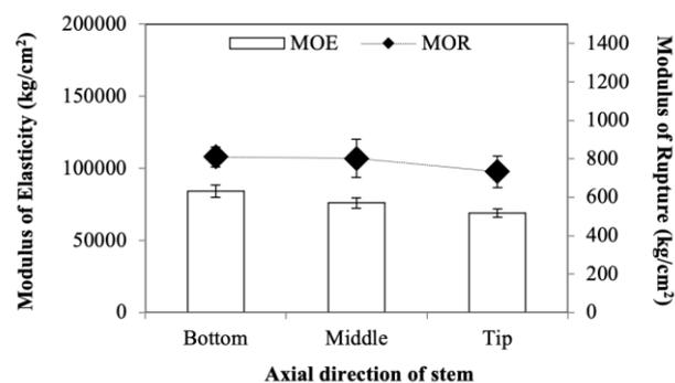
Figure 7. Modulus of elasticity and modulus of rupture Simalambuo wood
