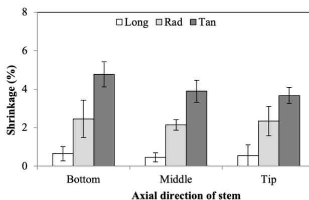
Figure 6. The shrinkage of Simalambuo wood
