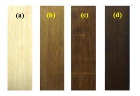
Figure 2. The look of jabon wood after being subjected to oil heat treatment at varying temperatures: (a) untreated sample, and heat-treated samples at (b) 170°C, (c) 190°C, and (d) 210°C
