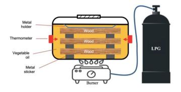
Figure 1. Oil heat treatment kiln
