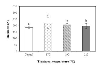
**Figure 6.** The temperature at which the oil is heated affects hardness of the jabon wood becomes (different letters above the bar graph show significantly different at a 5% confidence level)
