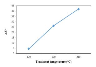
**Figure 4.** Change in  $\Delta E^*$  of jabon wood after oil heat treatment
