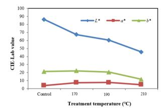
Figure 3. Change in  $L^*$ ,  $a^*$ , and  $b^*$  of jabon wood after oil heat treatment
