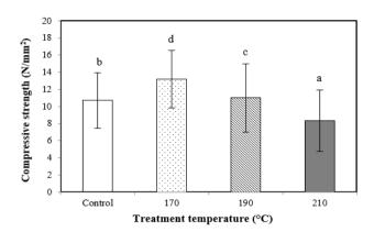
**Figure 5.** The temperature dependence of the increase in compressive strength of oil-heated jabon wood at various temperatures (different letters above the bar graph show significantly different at a 5% confidence level)
