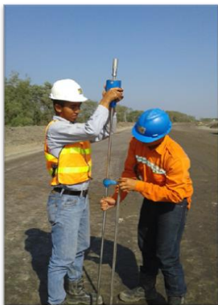
Gambar 3.5 Uji Dynamic Cone Penetration (DCP)
