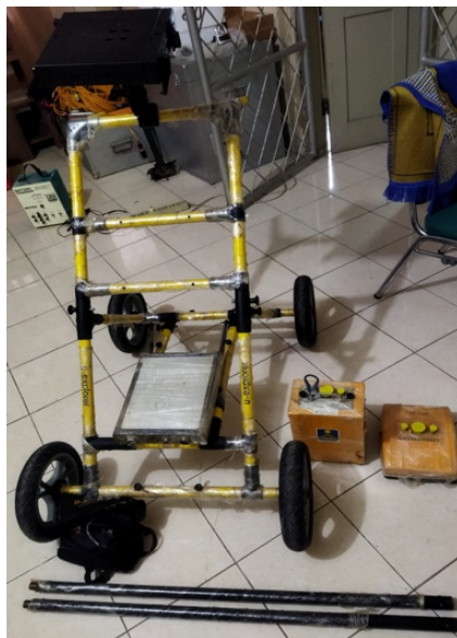
FIGURE 1. GPR body frame and 1GHz ground-coupled antenna
