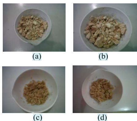
Figure 1. Visual Appearance of \text{Na}_2\text{CO}_3 Powder Produced at Different Concentrations of NaOH. (a) 6.5 M, (b) 7.0 M, (c) 7.5 M, and (d) 8.0 M
