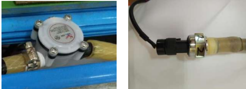
Gambar 6. Water flow meter dan pressure sensor
