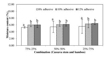
Figure 4. Effect of briquette combination and adhesive concentration on the moisture content of charcoal briquettes (different letters within a combination show significant different at a 5% significance level between adhesive content using Duncan's multiple-range tests)
