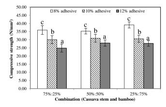
Figure 7. Effect of briquette combination and adhesive concentration on compressive strength of charcoal briquettes (different letters within a combination show significant different at a 5% significance level between adhesive content using Duncan's multiple-range tests)
