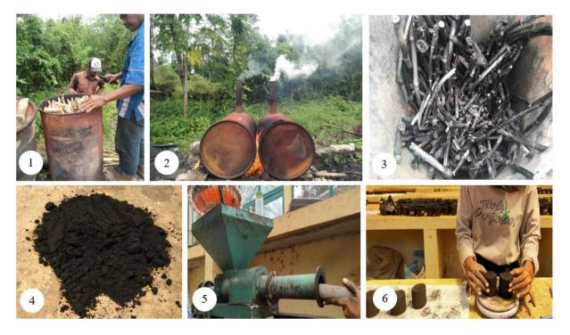
**Figure 2.** Stages of making charcoal briquettes. 1. Raw materials were put into the drum, 2. Process of coking cassava and bamboo sticks, 3. Results of coking, 4. Charcoal powder after grinding and sifting 40 mesh, 5. Briquette manufacturing, and 6. Finished and dried briquettes
