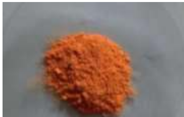
Figure 1. Synthesized Schiff base crystall solid
