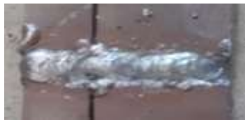
Figure 6. The welding results of 4.5 cm pre-heating distance
