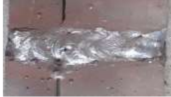
Figure 5. The welding results of 3 cm pre-heating distance
