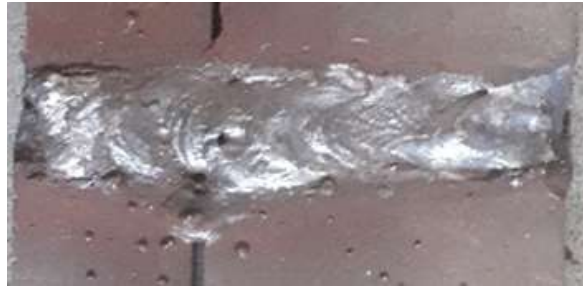
Figure 5. The welding results of 3 cm pre-heating distance
