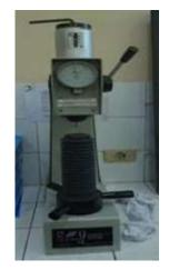
Figure 4. Hardness test equipment
